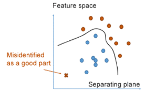
(a) Supervised machine learning (Separating plane learned using good and defective samples)
